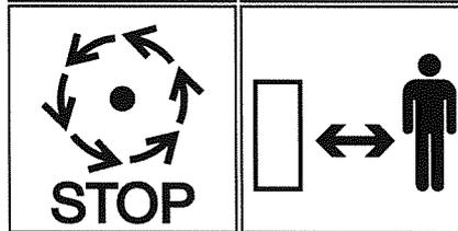
**Nr. 52**, Wait until all machine components have completely stopped before touching them. Stay clear of mower knife area as long as tractor engine is running with PTO connected.
