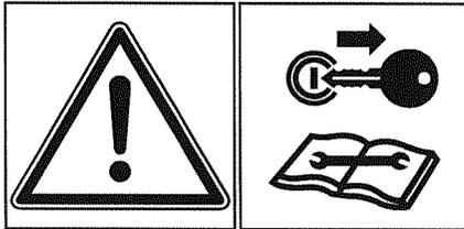
**Nr. 51**, Shut off engine and remove key before performing maintenance or repair work.
